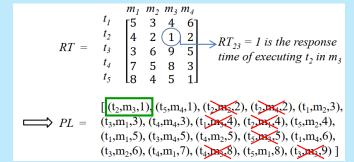
Iteration 2: Assign t<sub>5</sub> to m<sub>4</sub>
