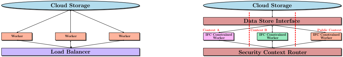
Fig. 4: A scalable webservice worker process design running multiple identical instances of an application. We reduce the attack surface by running the multiple instances in different security contexts.
