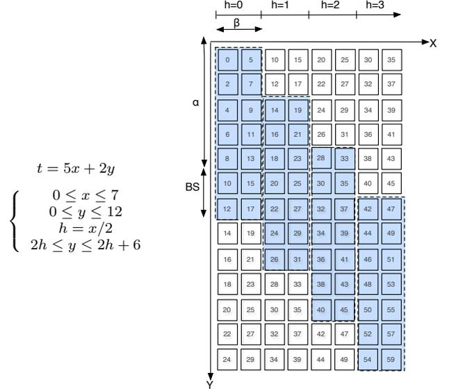
Fig. 10. Load-balanced cuts for redundancy elimination
