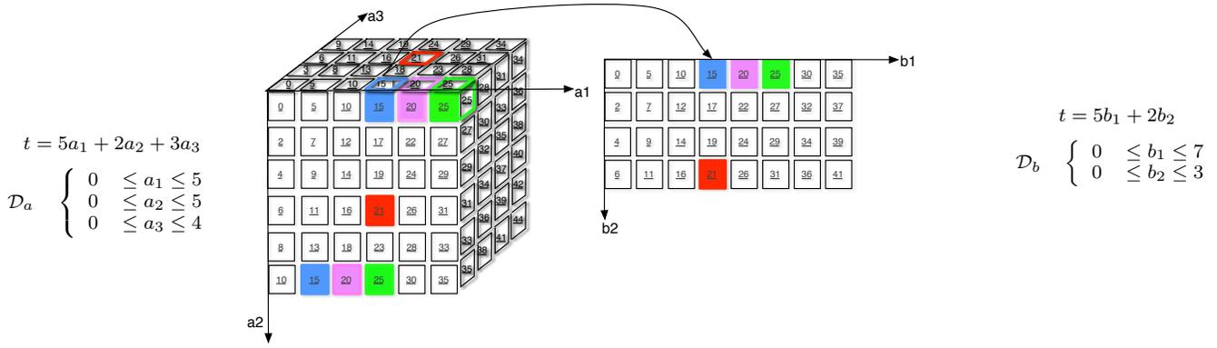
Fig. 5. Polyhedral representation of the source A and destination B distributions for a mono-dimensional array. For instance, the blue element  $t=15$ , of coordinates  $(3,0,0)$ , on the first row of A is mapped to  $t=15$ , of coordinates  $(3,0)$  in B.
