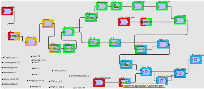
Fig. 3. Mapping the example application onto the example architecture. The application graph is partitioned into different coloured segments that work in a Kahn Process Network-like manner. Each segment is mapped onto a part of the architecture containing one or more processing elements intra/inter tile.
